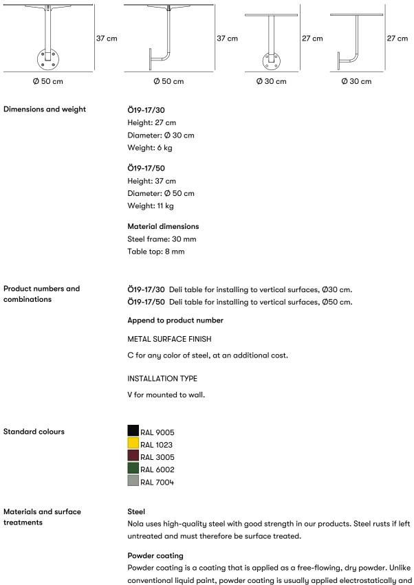
then cured under heat or with ultraviolet light. The result is an even, hard-wearing coloured surface with the desired gloss level.
