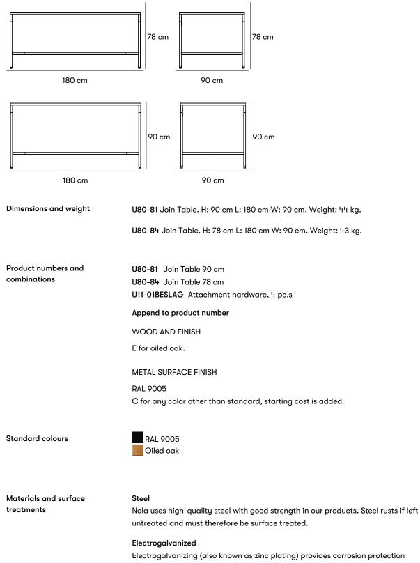
through the sacrifice of zinc ions. It is created via a zinc coating on the steel using an electric current.
