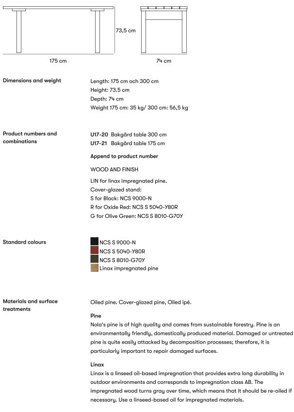
After traditional impregnation according to NTR AB, the wood is boiled in a hot linseed oil with or without color pigments under vacuum. The oil is penetrated into the surface on all six sides, which reduces moisture absorption in the wood and
